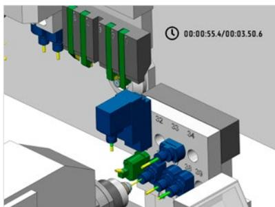
The calculated cycle time is displayed in the simulation module.
