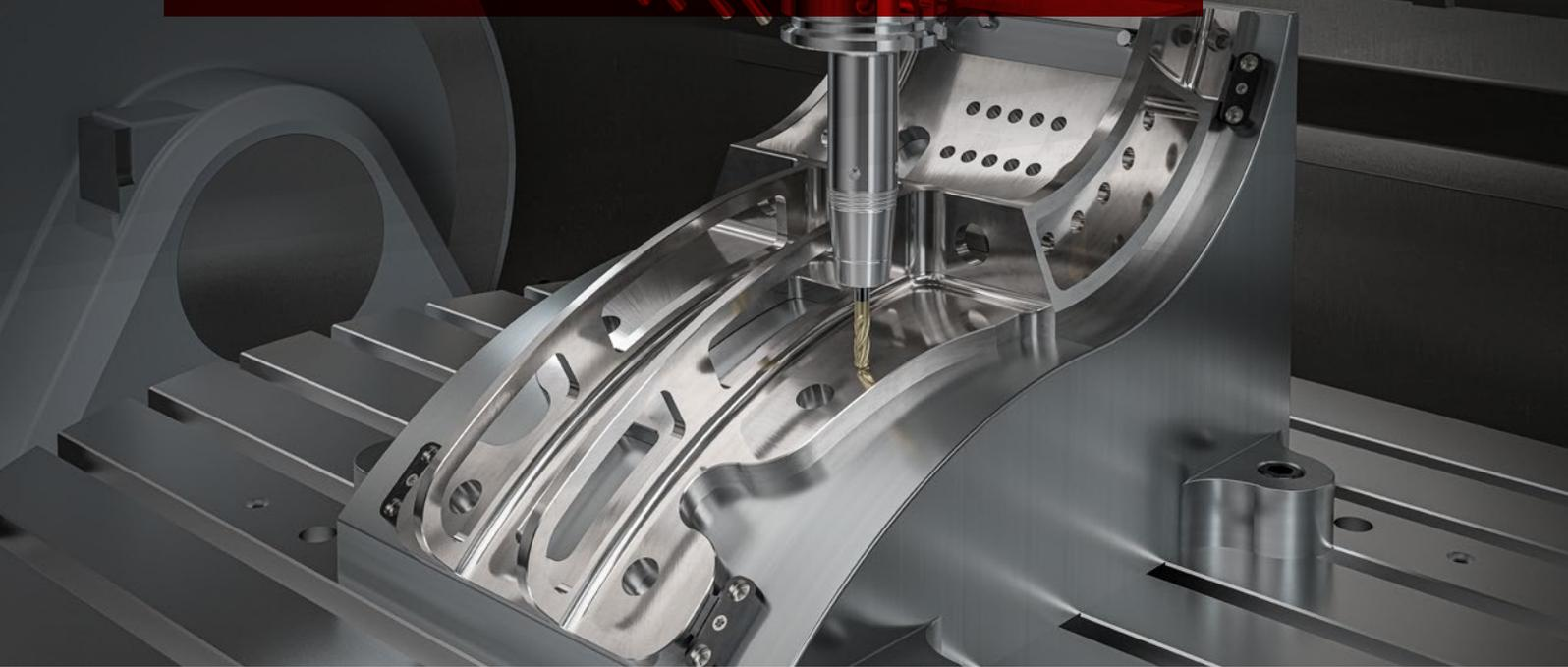
SolidCAM HSS is a high speed surface machining module for smooth and powerful machining of localized surface areas in the part, including undercuts. It provides easy selection of the surfaces to be machined, with no need to define the boundaries. It supports both standard and shaped tools.
