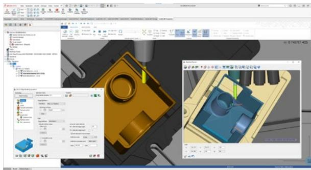
SolidCAM's Edge Breaking operation creates a deburring tool path on the outer edges of a part geometry. The position of the tool relative to the edge is always the bi-vector between the two surfaces of that edge.
