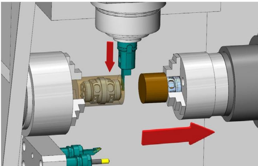
SolidCAM always keeps the stock updated live, within the operations tree, to optimize the tool-path, avoid air-cutting and to achieve minimal cycle time.
