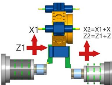
SolidCAM supports three different superimposition modes. A pair of axes can be superimposed one to another, where the slave one follows the master one.
