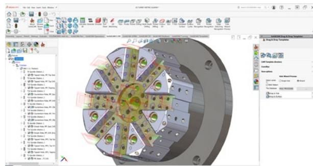
Drill features detection & Automatic Tool path generation
