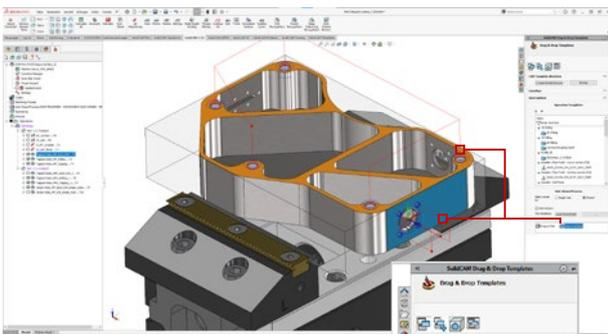
The new "Drag to Surface" function will create operations for all holes with the same coordinate system alignments.
