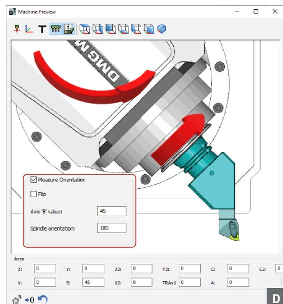
Measured tool orientation on spindle with tilt axis
