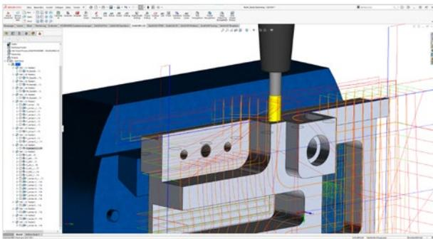
functions, SolidCAM's post processors are built to use these internal CNC functions. If you have a machine without such functions, users can input the part location inside SolidCAM and the G-code will handle all of the transformations for each rotation.
