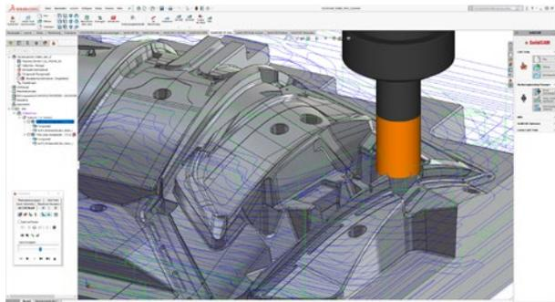
THSR and THSM offer unique machining and linking strategies for generating high-speed tool paths. The 3-Axis calculation engine recalculates the tool path at lightning speeds. Its 64-bit architecture completely utilizes all the cores for tool path calculations.
