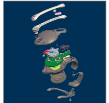
Logitech redesigned its headset to improve the microphone boom's strength.
