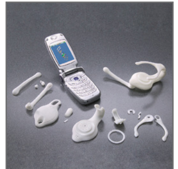
Headset components were modeled in ABS plastic, using the FDM process.
