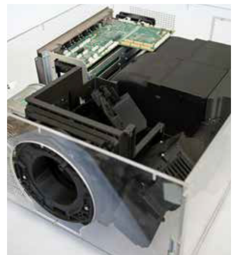
This mockup projector has a combination of 3D printed and production components.
