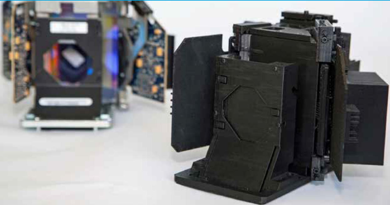
Light engine mock-up (right) and production unit
