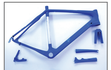
This complete bicycle frame used for functional testing was 3D printed with the Dimension 3D Printer.
