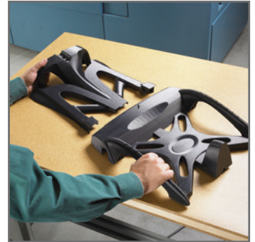
The carrier rack prototype was built in two pieces and assembled.
