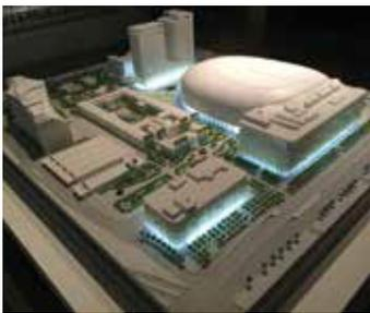
Professional model producer Transference improved its delivery speed of high-end models like this one by incorporating 3D printing into its design process.
