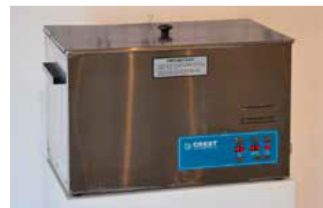
Supports on the parts are dissolved away in a tank filled with an alkaline-based solution.
