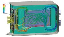
Using SolidWorks Flow Simulation software, ioSafe optimized the balance of air flow for cooling and outward steam flow during a fire.
