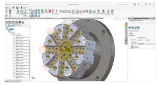
Drill features detection & Automatic Tool path generation
