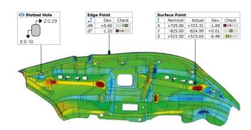
Benefit – With full-field component measurement, no spot remains unchecked. Easily understandable results instead of long tabular inspection reports enable a quick determination of correction values for tool geometry (springback, trimming) as well as for machine and process parameters (lubrication, down-holder forces, closing force ...).
