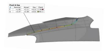
**Benefit** – Fast assembly analysis for prototypes, Meisterbock & Cubing as well as for series by real-time representation. Inspection of sub-assembly as well as of critical single parts (mounting geometries and component surface). Easy handling and low set-up requirements lead to the replacement of conventional gauges and fixtures.
