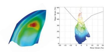
Benefit – Support for materials selection, evaluation of tools and optimization of process parameters of forming machines and forming processes. The verification of FE simulations based on measuring data serves for knowledge building and guarantees increased reliability of numerical simulations.
