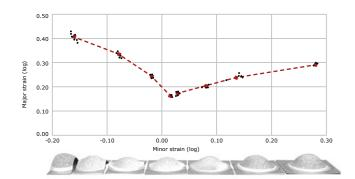
**Benefit** – Full-field measurements of material strain (major & minor strain) are substantially more accurate than determining by hand, magnifying glass or microscope. Reproducible determination of material properties for new alloys, incoming goods inspection and variations in quality within a coil.
